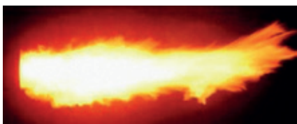
Conventional, strongly radiating, long oil flame producing soot.
