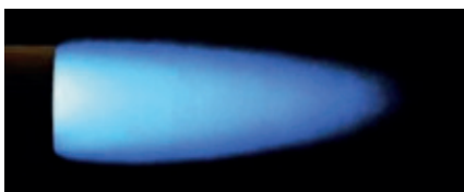
Bluish-transparent oil flame characteristic of the Ultramizing® combustion principle.
