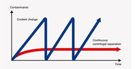
The blue sawtooth line shows how coolant that is not cleaned becomes progressively more contaminated to the point where total replacement becomes necessary. This will occur not once, but repeatedly. The red curve shows how a centrifugal separator maintains a constant low level of contaminants.
