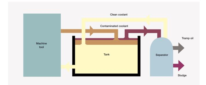
The separator operates continuously and requires no alterations to the existing installation.
