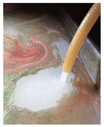
After cleaning, the coolant is returned to the tank.
